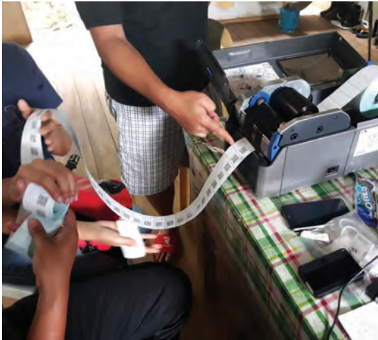
Lumber code: A machine in a lumber yard in Bukidnon prints out lumber QR code labels, which must be attached to each piece of lumber at the sawmill. Photo: FMB
